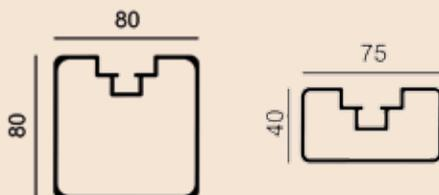
*Mini goals fully welded, post/crossbar made of profile 80 x 80 mm, ground frame made of aluminium profile 75 x 40 mm, in 3 different sizes.*
